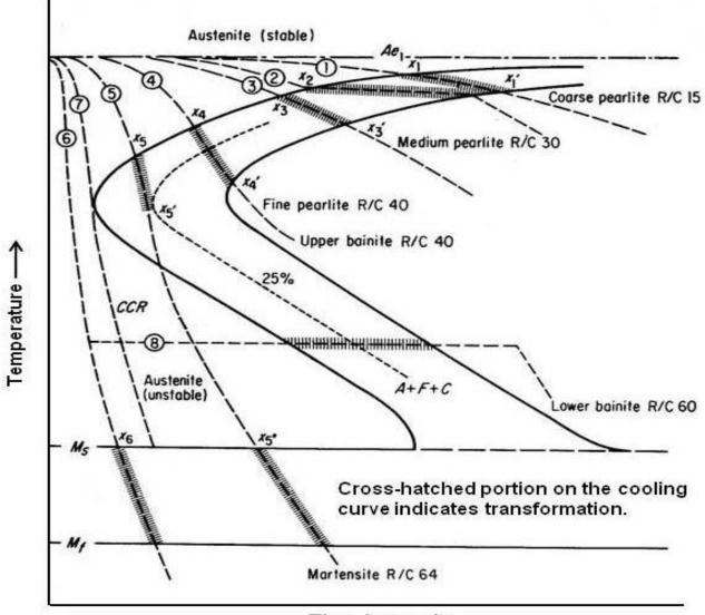
Time, log scale Cooling curves superimposed on a hypothetical I-T diagram
