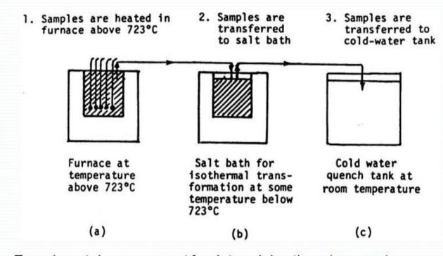
Experimental arrangement for determining the microscopic changes that occur during the isothermal transformation of austenite in an eutectoid plain-carbon steel
