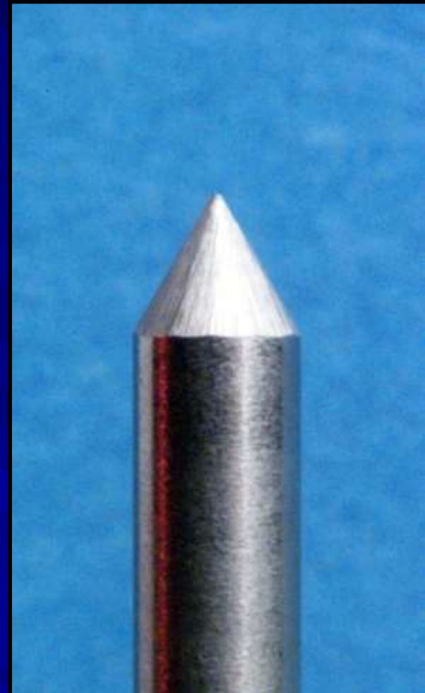
Electrode tip prepared for high current welding
