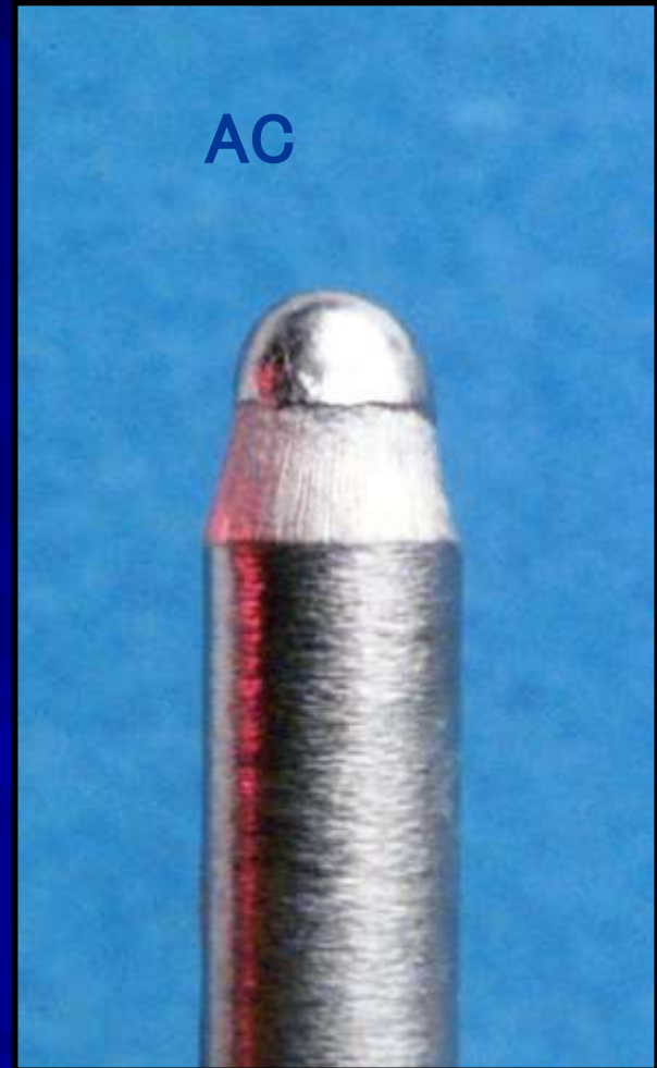
Electrode tip ground and then conditioned
