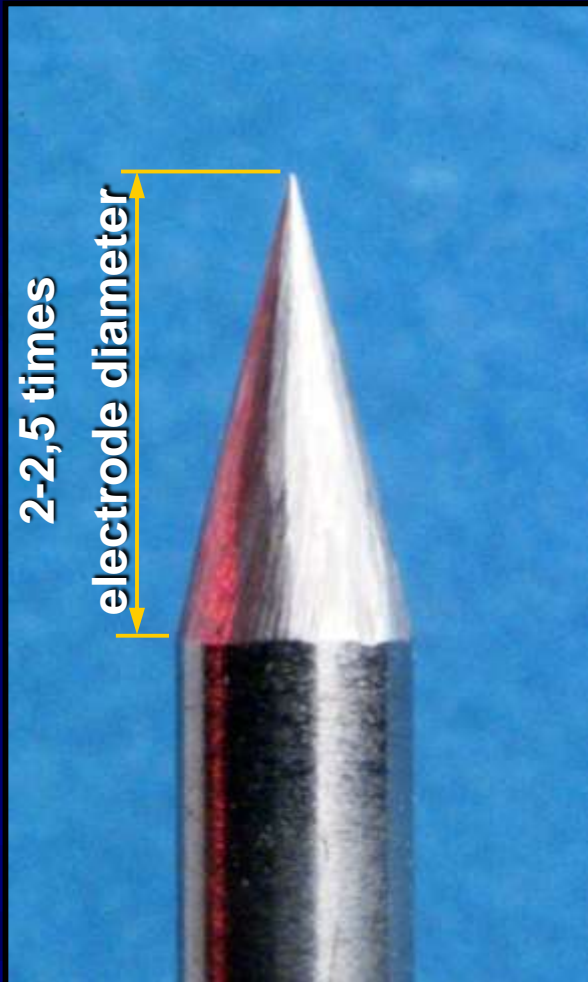
Electrode tip prepared for low current welding
