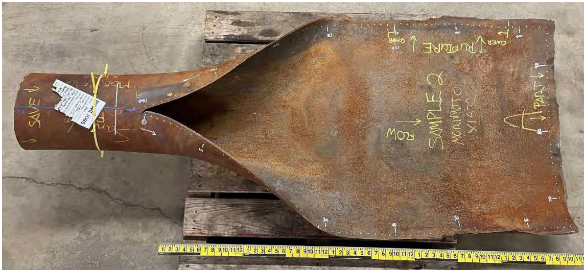
Figure 11. Ruptured tube. (Credit: PBF Energy)
