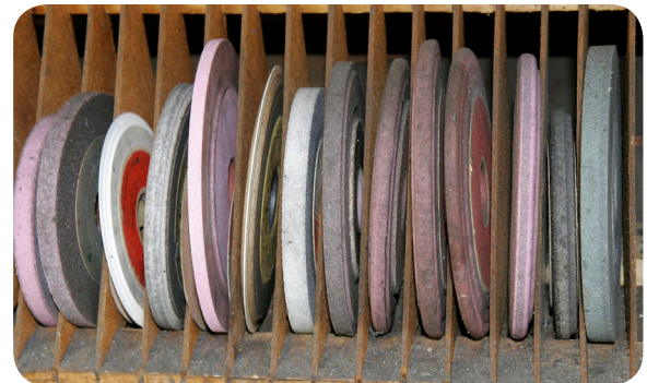
Abrasive wheels use grains to create friction between the wheel and the material to be sanded, polished, and/or buffed
