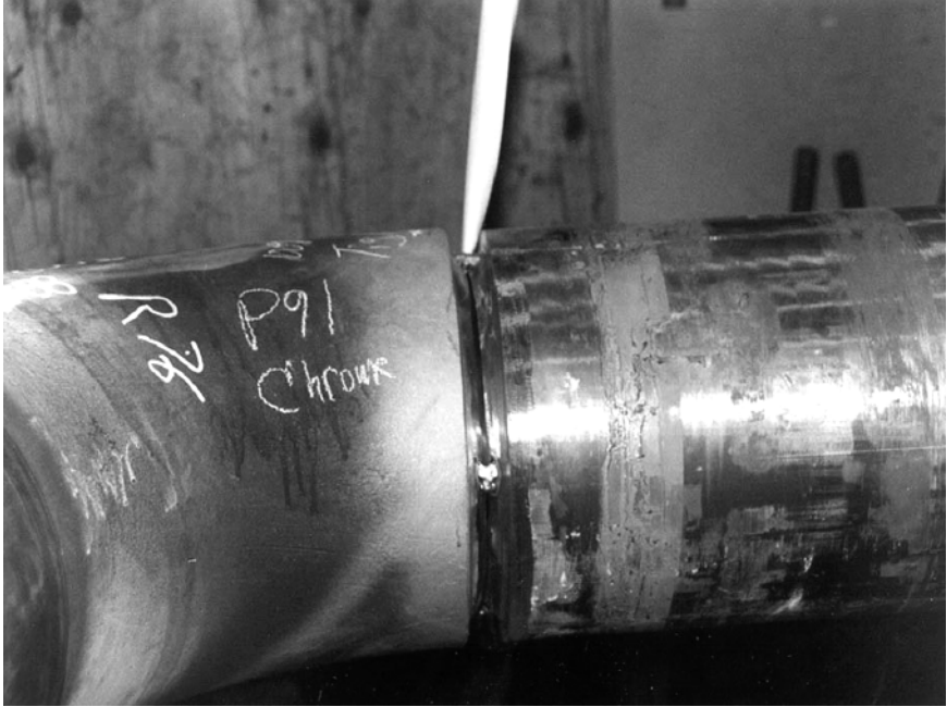
Figure 9.1 Weld fit-up and gap examples. (Photograph courtesy of TEAM Industries, Inc., Kaukauna, WI.)
