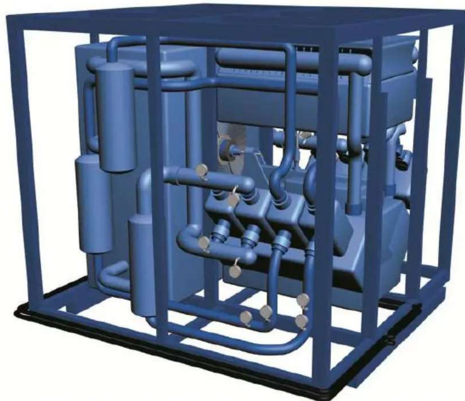
DIESEL ENGINE, USUALLY INSIDE SOUND-SUPPRESSED SYSTEM
