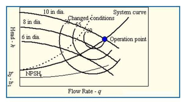
**Note**: The available NPSHa of the system should always exceed the required NPSHr of the pump to avoid vaporization and cavitation of the impellers and pump inner walls. The NPSHa is also calculated to avoid that head loss in the suction pipe and in the pump casing, local velocity accelerations and pressure decreases, start boiling the fluid on the impeller surface.
