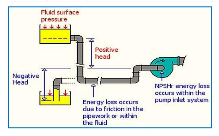
Note: See the tables indicating the energy loss due friction for water flow through ASME/ANSI B36.10 schedule 40 steel piping and fittings. The friction loss can be also calculated by, f (loss) =  $K \times v^2/2g$  ( $g = 32.17 \text{ ft/s}^2$ ).
