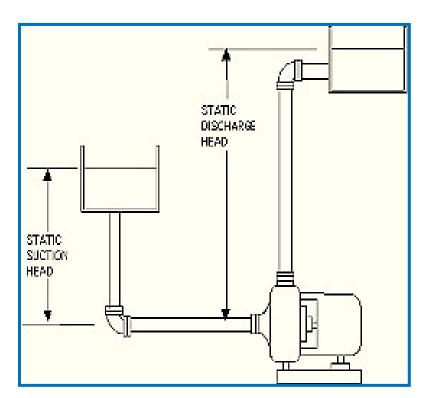
NPSHa = Static head + Atmospheric pressure (converted to head) + Vapor pressure of the fluid (converted to head) – Friction loss (in the piping, valves and fittings);
